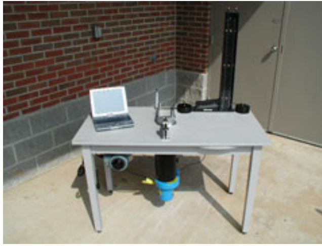
Frazier 2000 Electronic High Pressure Air Permeability Instrument
